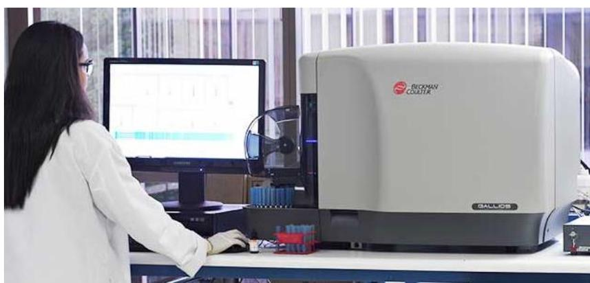
**Figura 2.23.** Gallios (Beckman Coulter). 2 lasers, 8 cores; Kaluza software. Foto: Beckman Coulter.
