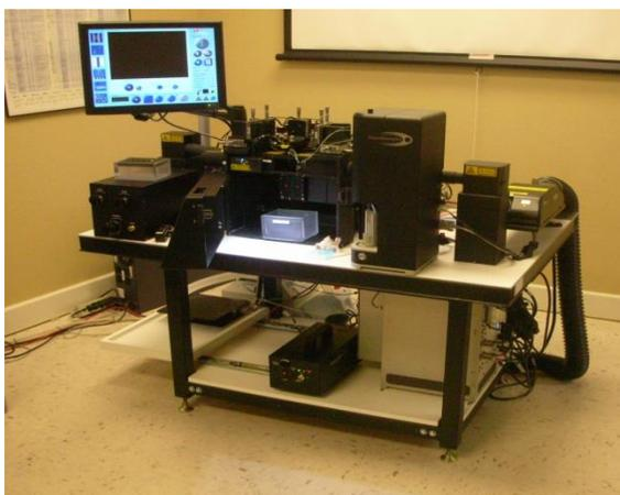
**Figura 2.26.** MoFlo XDP *Cell Sorter* (Beckman Coulter). 3 *lasers*, 11 *cores*. *Software*: Summit 5.0.
