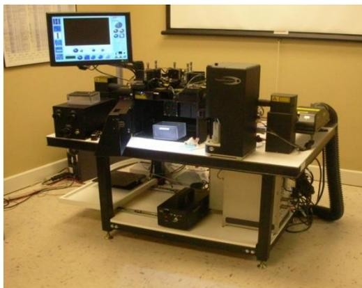
**Figura 2.29** - MoFlo XDP *Cell Sorter* (Beckman Coulter). 3 LASERs, 11 cores. Software: Summit 5.0.
